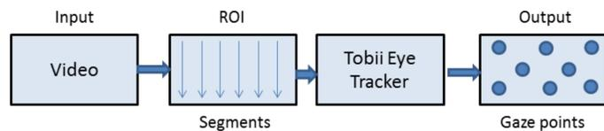
Figure 1: Block Diagram of Eye-Tracking based RoI Detection
